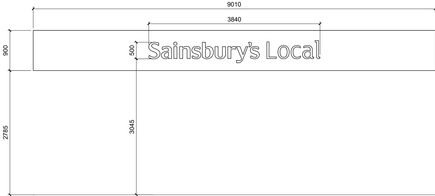
04 PROPOSED FASCIA SIGNAGE C-INTERNALLY ILLUMINATED- P129423213 1:50@A3 ILLUMINATION LEVEL - 375 cd/m²
