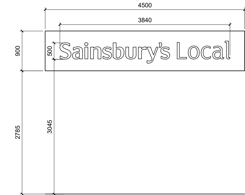
01 PROPOSED FASCIA SIGNAGE A -INTERNALLY ILLUMINATED- P129423213 1:50@A3 ILLUMINATION LEVEL - 375 cd/m²
