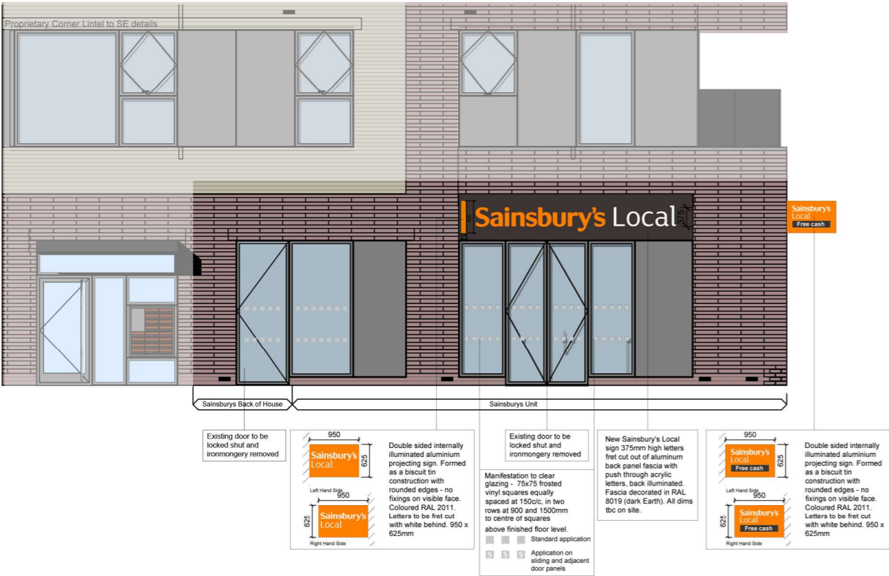
02 PROPOSED SIDE ELEVATION 1:125 @ A3
